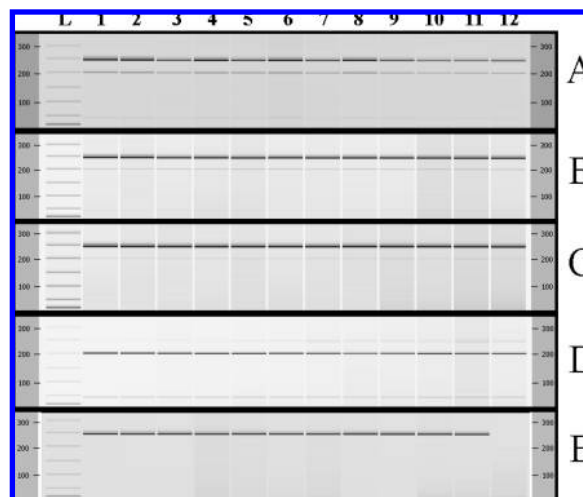
Figure 4. Electropherograms of digested samples from grapevine must mixtures during fermentation. (A) Agiorgitiko:Cabernet (50:50), (B) Agiorgitiko:Cabernet (75:25), (C) Agiorgitiko:Cabernet (90:10), (D) Cabernet (100%), and (E) Agiorgitiko (100%). The fermentation days of the samples from A to D are as follows: 1–2, third day; 3–4, fourth day; 5–6, fifth day; 7–8, sixth day; 9–10, seventh day; and 11–12, eighth day. Lane: L, DNA ladder. For E, the fermentation days are as follows: 1–2, 0 day; 3, third day; 4, fifth day; 5, sixth day; 6, seventh day; 7, eighth day; 8–9, 0 day prior to digestion; 10, seventh day prior to digestion; and 11, eighth day prior to digestion.
